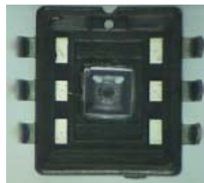
Fig. 1 The conventional DIP packaging pressure sensor Reference: NAIS, ADP1131
